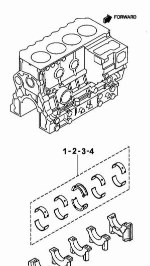
Section: B0 - ENGINE MAIN BEARINGS
