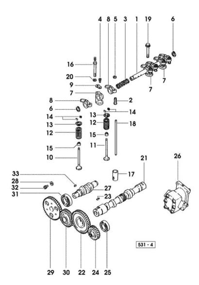
Section: ENGINE CAMSHAFT
