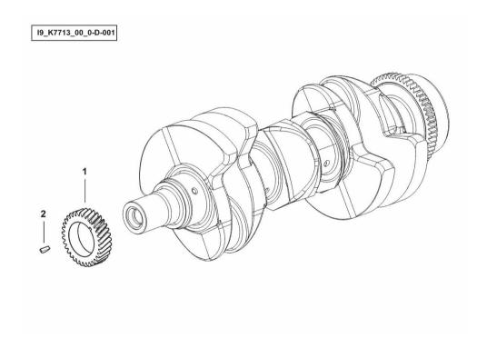
Section: B0 - ENGINE CRANKSHAFT GEAR
