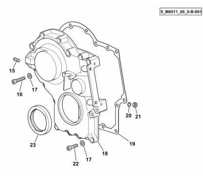
Section: B0 - ENGINE TIMING CASE
