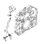
Section: B0 - ENGINE **BLEEDING TUBE**
