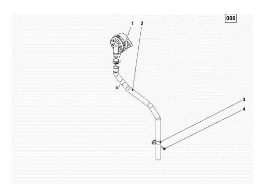
Section: B0 - ENGINE **BLEEDING TUBE**
