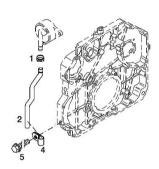
Section: B0 - ENGINE **BLEEDING TUBE**
