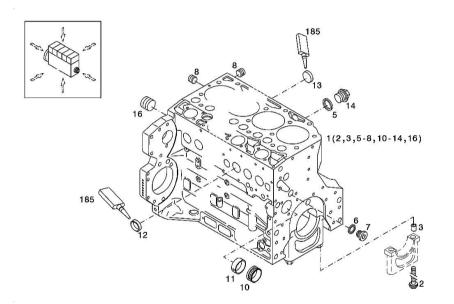
Section: B0 - ENGINE CRANKCASE
