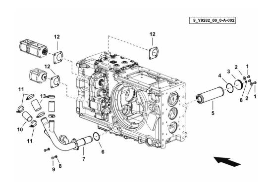
Section: H0 - HYDRAULIC AND PNEUMATIC SYSTEM SUCTION HYDRAULIC SYSTEM 16+22,5+14 CC
