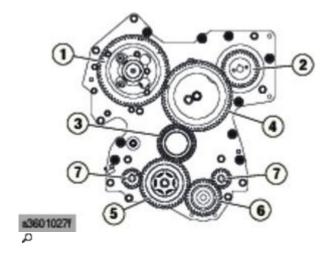
On a **4-cylinder** engine, set the timing of the balancer shafts (7) and lower intermediate pinion (5).
