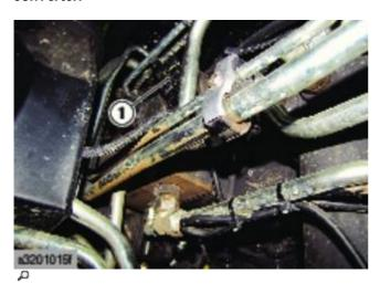
▶ If fitted, disconnect and detach the connector (1) used to control the front loader.
