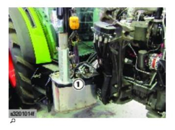
▶ Sling and remove the "SCR" catalytic converter assembly and its support and the booster foot using a suitable lifting tool.
