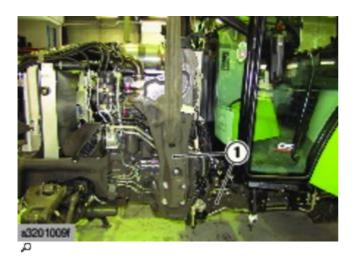
► If fitted, remove the bracket and side member (1) from the loader frame on the left-hand side using a suitabl lifting tool.
