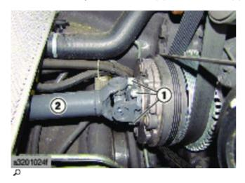
▶ Remove the bolts (1) of the front power take-off drive flange (optional).
