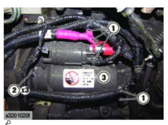
▶ Remove the protective panel from the electric starting motor.
