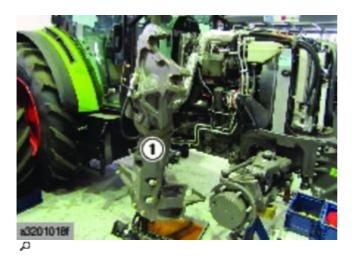
▶ If fitted, remove the bracket, side member and cross member (1) from the loader frame on the right-hand side using a suitable lifting tool.
