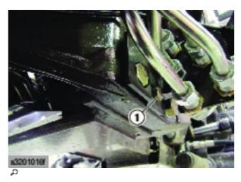
▶ If fitted, remove the bolt (1) mounting the pipe support to the front loader.
