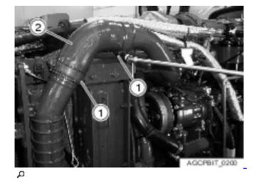
► Remove the clamps (1) and remove the sleeve (2).
