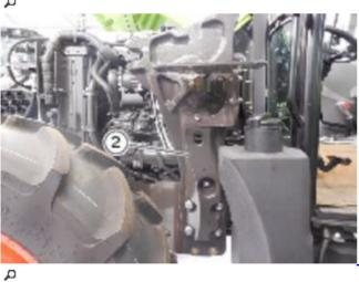
▶ If fitted, remove the loader brackets (1 and 2) from the loader frame using a suitable lifting tool.
