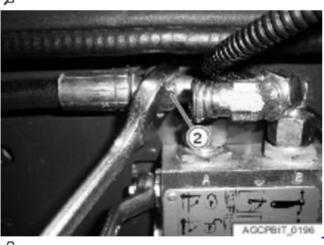
▶ Position a suitable container underneath the front linkage adjustment valve then disconnect the hoses (1 and 2).
