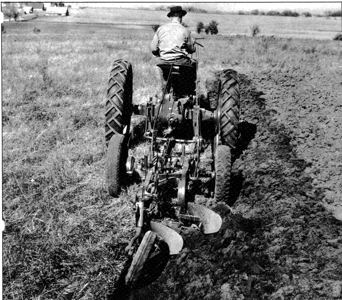
Two-furrow plow (clutch type lift) with pneumatic tires shown with the Farmall H Tractor.
