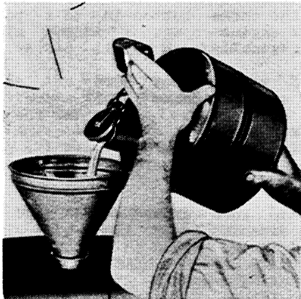
Illust. 7 - Filling the Fuel Tank.
