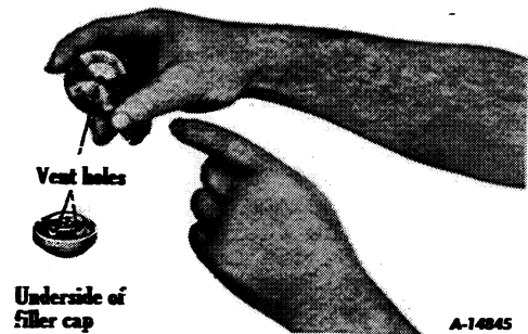
Illust. 8 - Vent Holes in Filler Cap.
