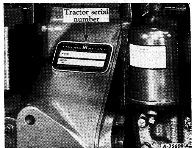
Illust. 3A Location of tractor serial number.
