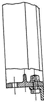
No. 1. Position of Front Wheel Skid Rings for Flat Ground Operation.
