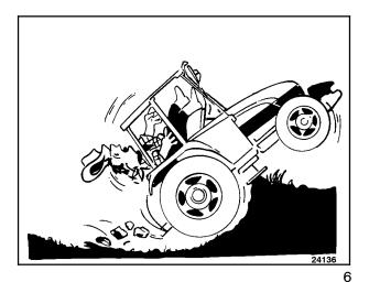
21. Engage the clutch slowly: if engaged too quickly, especially when the tractor is getting out of a hole, ditch or operating on muddy ground or steep slopes, the tractor may overturn.
