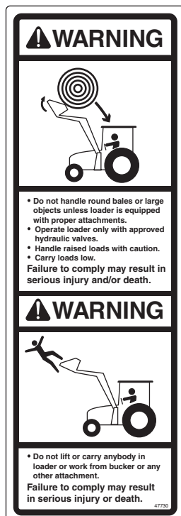
⑤ WARNING Decal Part No. 86581706 Location: Loader Left Side Frame Upright
