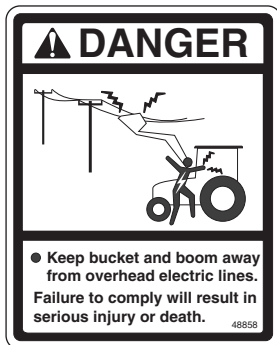
④ DANGER Decal Part No. 86583639 Location: Backside Loader Left Side Frame Upright
