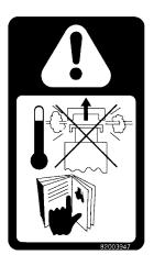
Warning! Pressurized cooling system. Allow to cool then remove cap carefully. Using a cloth, turn cap to the first stop and allow pressure to subside before removing cap completely.
