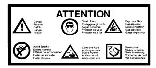
Danger! Corrosive acid. Explosive gas. Wear eye protection. Avoid producing sparks. See Operator's Manual.
