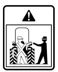
To avoid injury, do not stand on the implement or between the implement and tractor while making adjustments or connecting/disconnecting implements.
