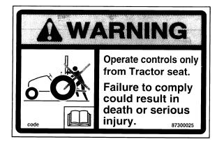
WARNING: Operate Controls only from Tractor seat PART NO: 87300025 LOCATION: Rear of Right and Left Fenders
