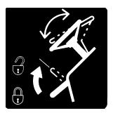
Steering Wheel Tilt PART NO: SBA390198970 LOCATION: Left side of steering column shroud
