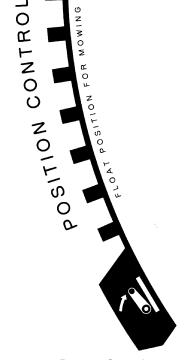
Position Control Lever PART NO: SBA390372490 LOCATION: Right Side Fender
