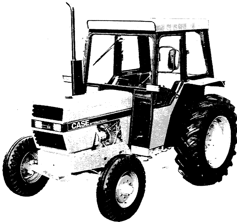
248L 2WD TRACTOR WITH A NON ADJUSTABLE, CAST FRONT AXLE AND A FABRICATED FRONT BOLSTER
