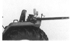
**IMPORTANT:** When the ROPS frame is in the lowered position, make sure there is clearance between the frame and hitch mounted equipment. Slowly raise the hitch to maximum height to check for necessary clearance. For drawbar attached and/or PTO driven equipment, check for clearance including turning corners.
