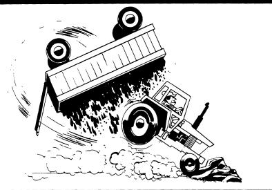
WARNING Tractor travel speed should be such that complete control and tractor stability is maintained at all times. Where possible, avoid operating the tractor near ditches, embankments and holes. Reduce speed when turning, crossing slopes, and on rough, slick, or muddy surfaces.
