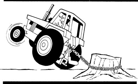
**WARNING** Extreme care must be exercised when adjusting and checking hitch and control linkage when the engine is running and when linkage is under hydraulic or mechanical load. Study the linkage and hitch travel-Keep the hands, arms, legs and feet out of the travel arc of the hitch and linkage.
