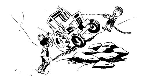
**WARNING** Stay off slopes too steep for safe operation. Shift down before you start up or down a hill with a heavy load. Avoid "free wheeling".
