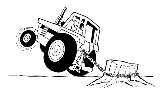
Try to balance the load primarily on the implement wheels - as in loading a trailer or spreader. Avoid overloading the drawbar. Add front end weights for improved stability. Engage the clutch smoothly, avoid jerking and use the brakes cautiously to avoid jack-knifing.
