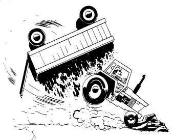
Brake pedals' must be locked together for road travel. This will insure uniform brake application and maximum stopping ability.
