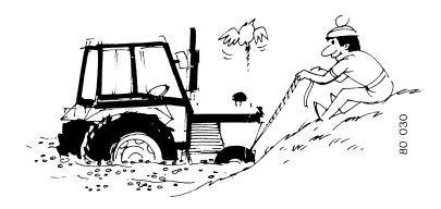
WARNING: Rear upset can result if pulling from wrong location on tractor. Hitch only to the drawbar. Use 3 point hitch only with the implements designed for its use — not as a drawbar.
