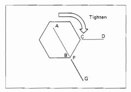
7. Use a socket wrench to tighten each nut or bolt to the point where the line [A-B] is aligned with the line [F-G].
