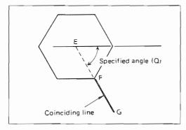
6. Draw another line [F-G] on the face of each of the parts to be clamped. This line will be in the direction of the specified angle [Q] across the center [E] of the nut or bolt.
