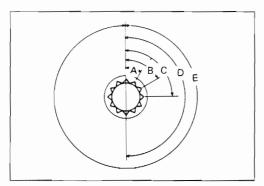
Example: Specified Angle and Tightening Rotation
