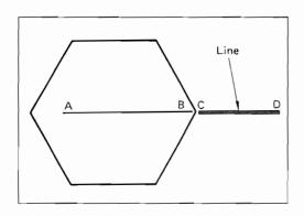
5. Draw another line [C-D] on the face of each of the parts to be clamped. This line should be an extension of the line [A-B].
