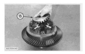
13. Remove gear (15) from the spider gears.
