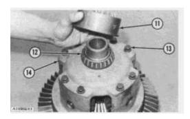
**10.** Remove small cage (11) from the differential. Remove the nut and the bearing cup from the cage.
