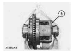
**8.** Fasten a hoist and a strap to the differential (9) as shown. Lift the differential and remove it from the carrier. Weight is 240 lb. (109 kg).
