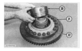
19. Remove cage (20). Remove the nut, the bearing cup, the ring and the two seals from cage (20).
