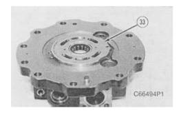
19. Reposition the travel brake valve body as shown. Remove plate (33) from the body.
