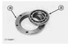
1. Install bearing (22) in carrier (23).
