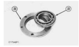
10. Remove bearing (22) from carrier (23).
