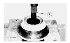
**8.** Use tooling (A) and a press to remove the bearing from the cage.
