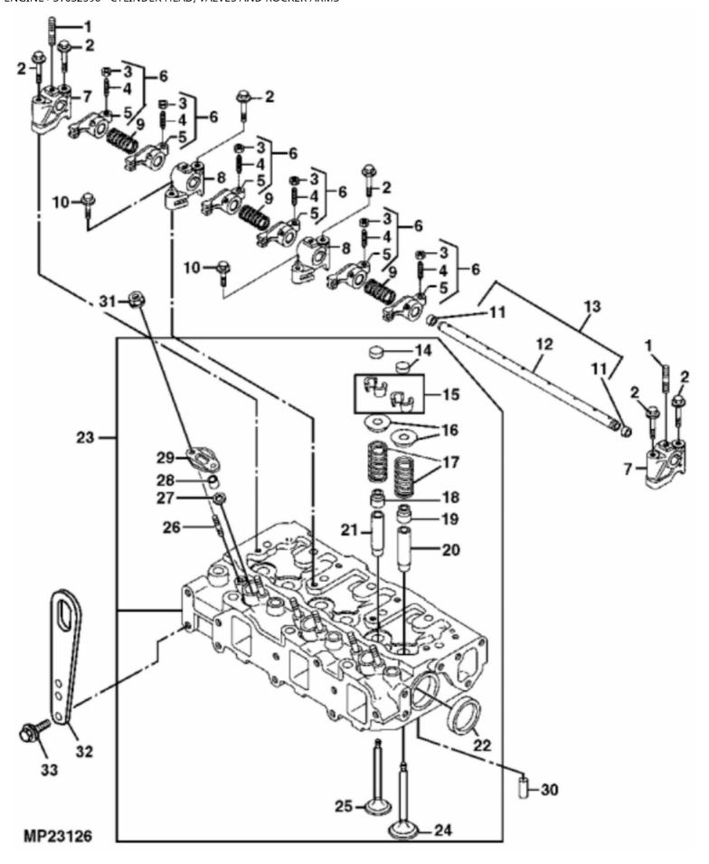
John Deere > Turf And Utility >TRACTOR, COMPACT UTILITY >4300 - TRACTOR, COMPACT UTILITY >4300 Compact Utility Tractor >20 ENGINE >ST632590 - CYLINDER HEAD, VALVES AND ROCKER ARMS
