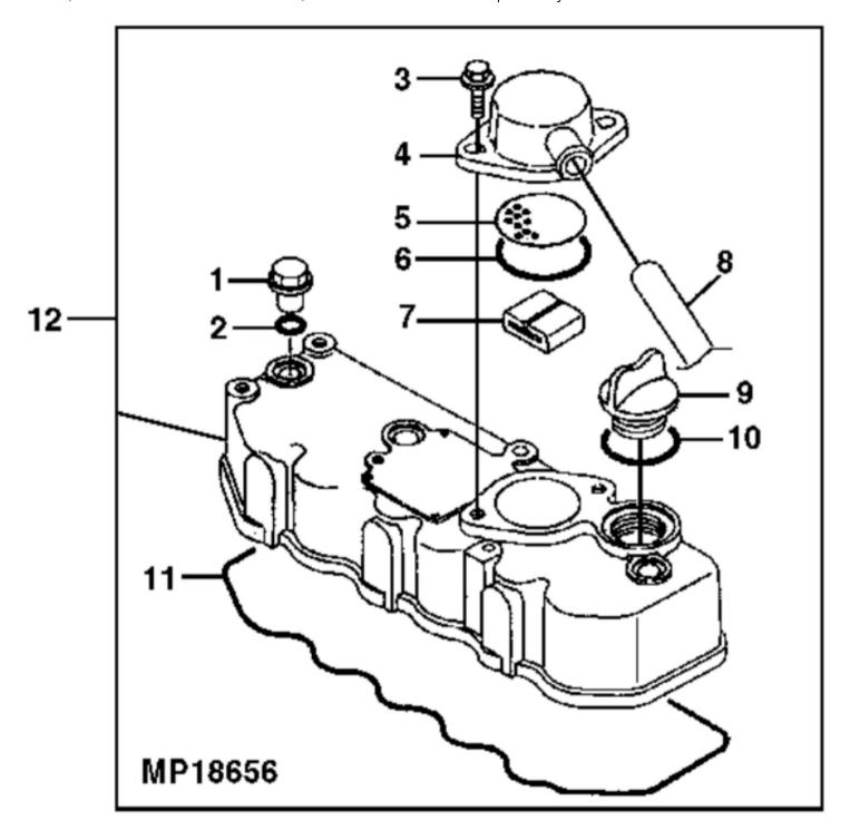
John Deere > Turf And Utility >TRACTOR, COMPACT UTILITY >4300 - TRACTOR, COMPACT UTILITY >4300 Compact Utility Tractor >20 ENGINE >ST632591 - CYLINDER HEAD COVER AND GASKETS
