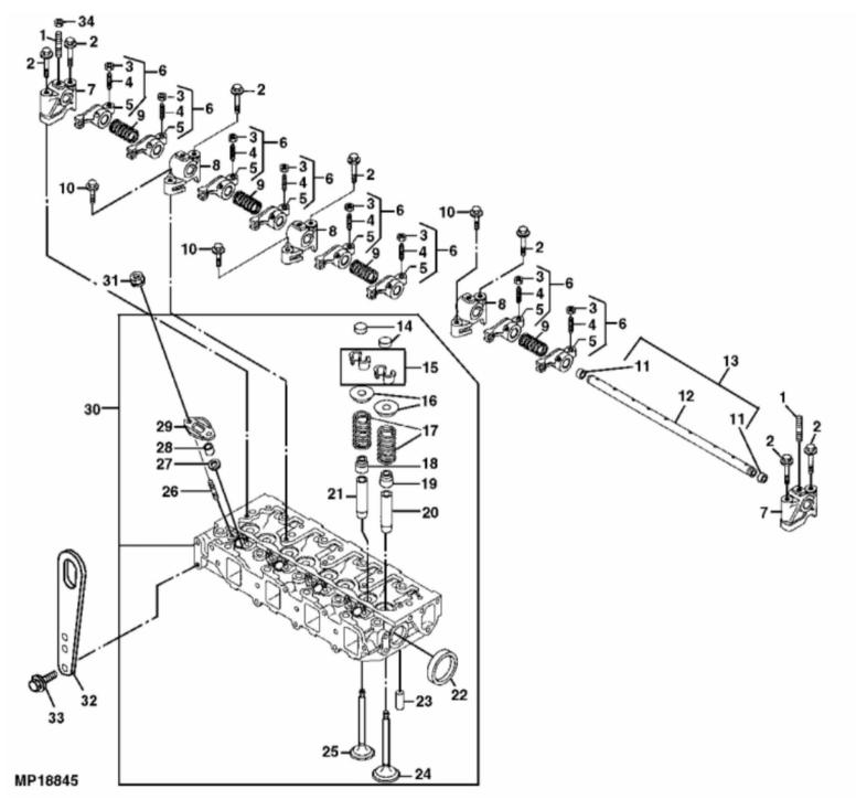
John Deere > Turf And Utility >TRACTOR, COMPACT UTILITY >4TNE88 - TRACTOR, COMPACT UTILITY >4700 Compact Utility Tractors >20 ENGINE >ST633056 - CYLINDER HEAD, VALVES AND ROCKER ARMS
