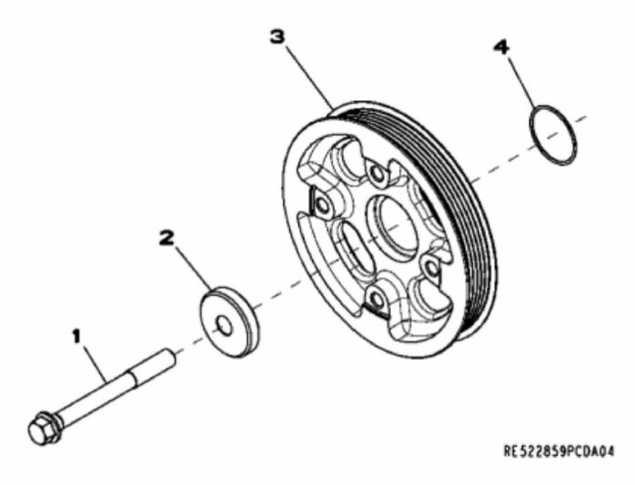
John Deere > Turf And Utility >TRACTOR >5065M - TRACTOR >5065M Tractor (Engine 5030HLV11)(IT4)(North America Edition) >23 ENGINE 5030HLV11 >ST435747 - 1303 CRANKSHAFT PULLEY
