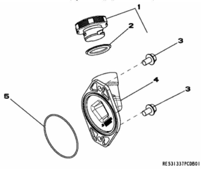
John Deere > Turf And Utility >TRACTOR >5075M - TRACTOR >5075M Tractor (Engine 5030HLV11)(IT4)(North America Edition) >23 ENGINE 5030HLV11-RE558558 >ST708086 - 1203 OIL FILLER NECK
