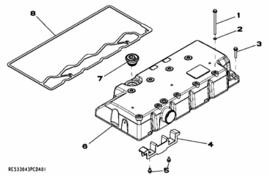
John Deere > Turf And Utility >TRACTOR >5075M - TRACTOR >5075M Tractor (Engine 5030HLV11)(IT4)(North America Edition) >23 ENGINE 5030HLV11-RE558558 >ST299045 - 1115 ROCKER ARM COVER
