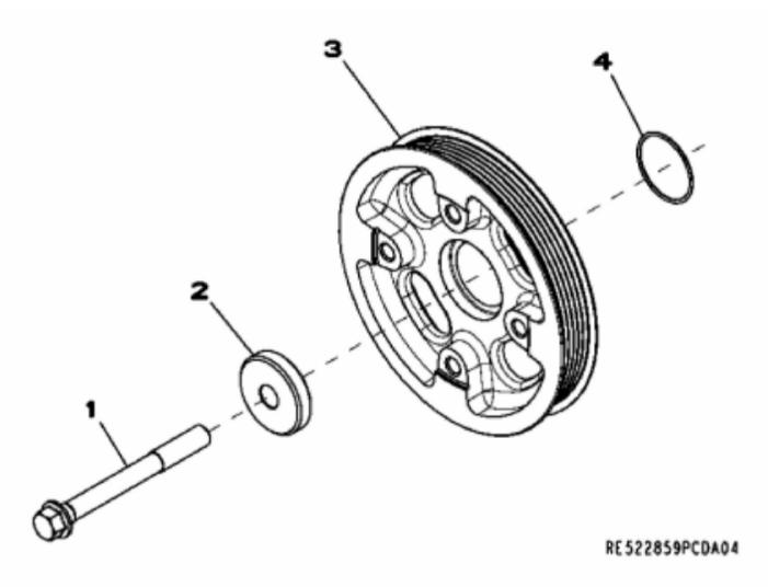
John Deere > Turf And Utility >TRACTOR >5075M - TRACTOR >5075M Tractor (Engine 5030HLV11)(IT4)(North America Edition) >23 ENGINE 5030HLV11-RE558558 >ST435747 - 1303 CRANKSHAFT PULLEY
