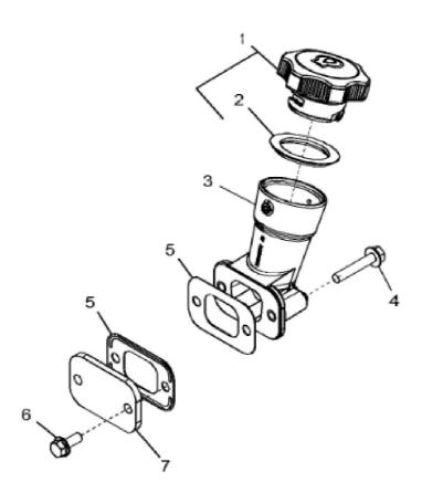
John Deere > Turf And Utility >TRACTOR >5085M - TRACTOR >5085M Tractor (Engine 4045HLV53,4045HLV54)(Tier 3)(Worldwide Edition) >23 ENGINE 4045HLV53 >ST308623 - 1202 OIL FILLER NECK
