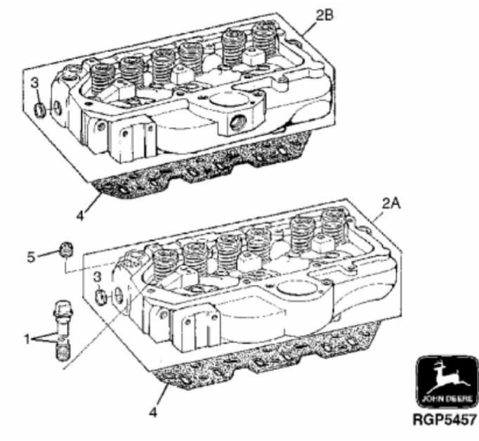
John Deere > Turf And Utility >TRACTOR >5400 - TRACTOR >5400N Tractor >20 ENGINE CD3029TLV01 >ST435307 - CYLINDER HEAD
