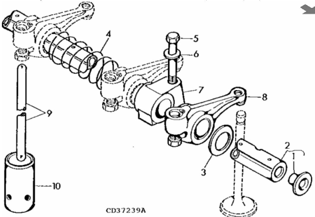
John Deere > Turf And Utility > TRACTOR > 5400 - TRACTOR > 5400N Tractor > 20 ENGINE CD3029TLV01 > ST435306 - ROCKER ARM / ROCKER ARM SHAFT / TAPPET / PUSH ROD
