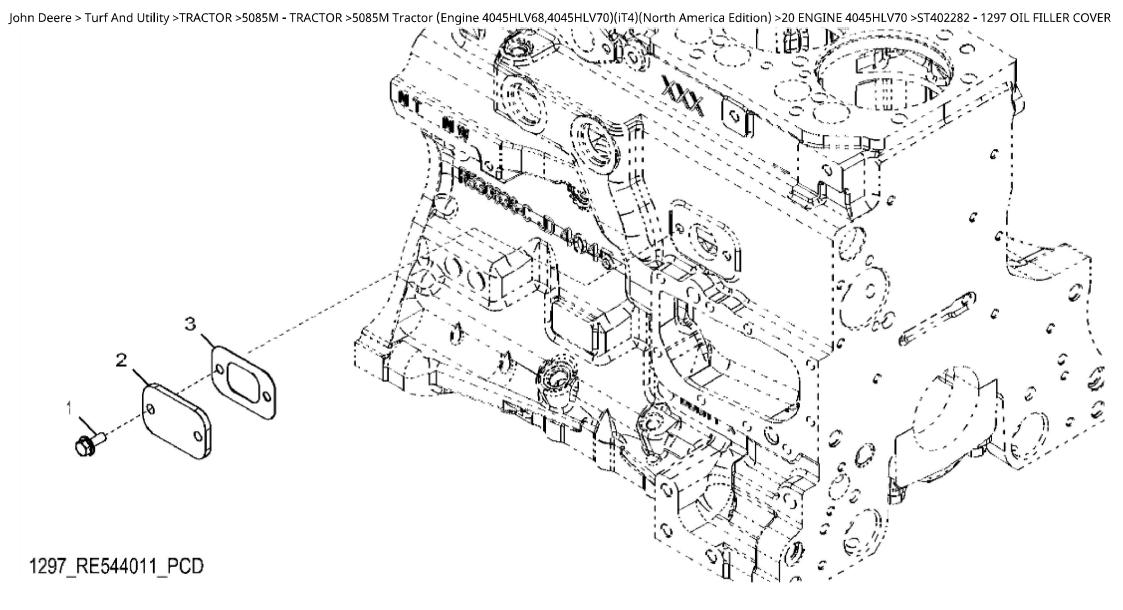
John Deere > Turf And Utility > TRACTOR > 5085M - TRACTOR > 5085M Tractor (Engine 4045HLV68,4045HLV70)(iT4)(North America Edition) > 20 ENGINE 4045HLV70 > ST402282 - 1297 OIL FILLER COVER
