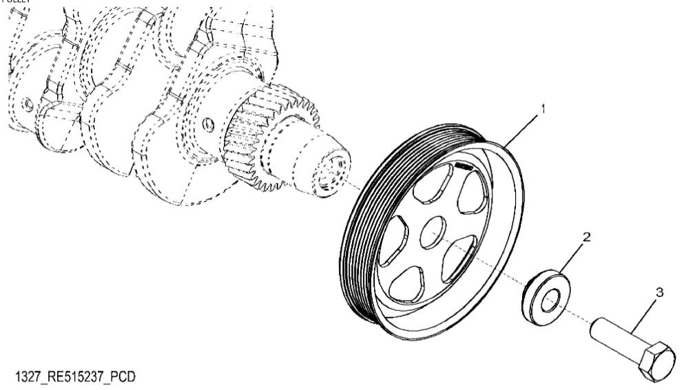
John Deere > Turf And Utility >TRACTOR >5085M - TRACTOR >5085M Tractor (Engine 4045HLV68,4045HLV70)(iT4)(North America Edition) >20 ENGINE 4045HLV70 >ST308624 - 1327 CRANKSHAFT PULLEY
