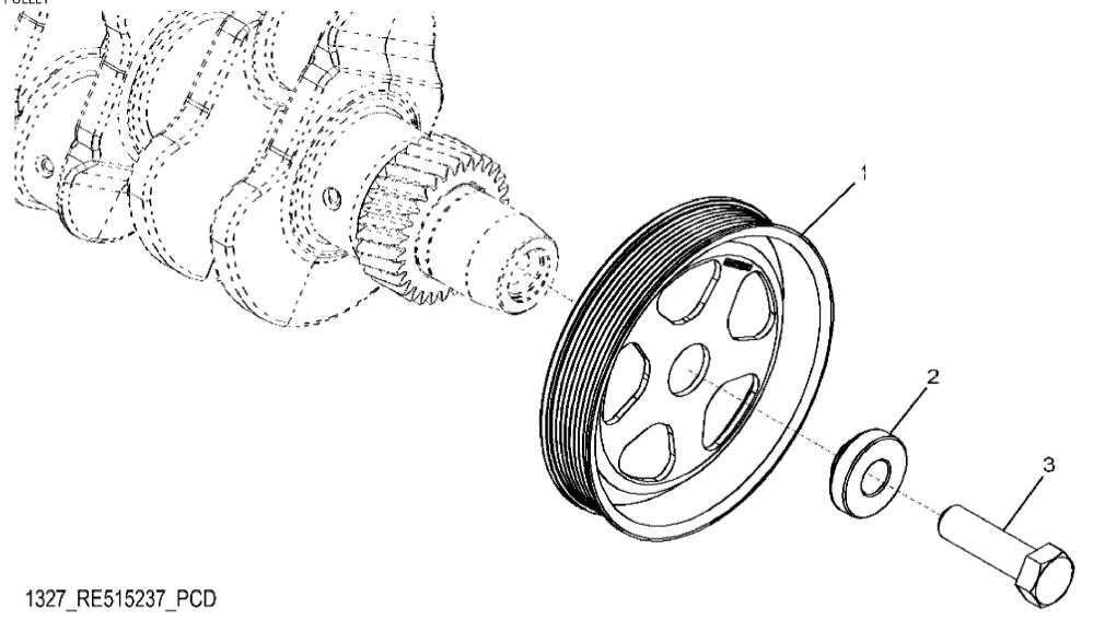
John Deere > Turf And Utility >TRACTOR >5100M - TRACTOR >5100M Tractor (Engine 4045HLV68,4045HLV70)(iT4)(North America Edition) >20 ENGINE 4045HLV70 >ST308624 - 1327 CRANKSHAFT PULLEY
