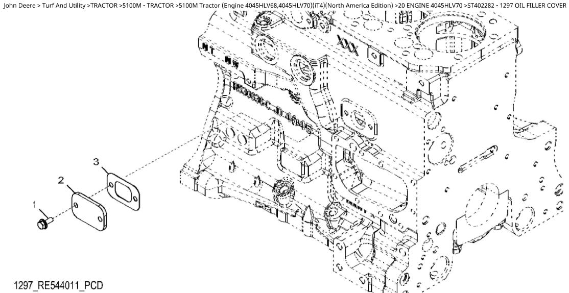
John Deere > Turf And Utility > TRACTOR > 5100M - TRACTOR > 5100M Tractor (Engine 4045HLV68,4045HLV70)(iT4)(North America Edition) > 20 ENGINE 4045HLV70 > ST402282 - 1297 OIL FILLER COVER
