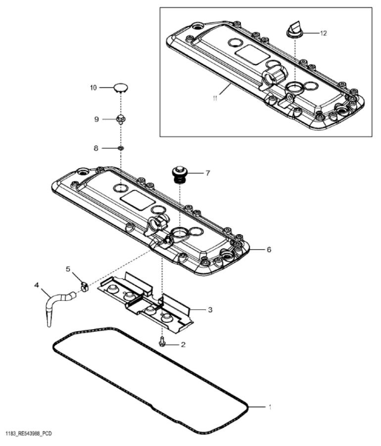
John Deere > Turf And Utility >TRACTOR >5100M - TRACTOR >5100M Tractor (Engine 4045HLV68,4045HLV70)(iT4)(North America Edition) >20 ENGINE 4045HLV70 >ST400926 - 1183 ROCKER ARM COVER
