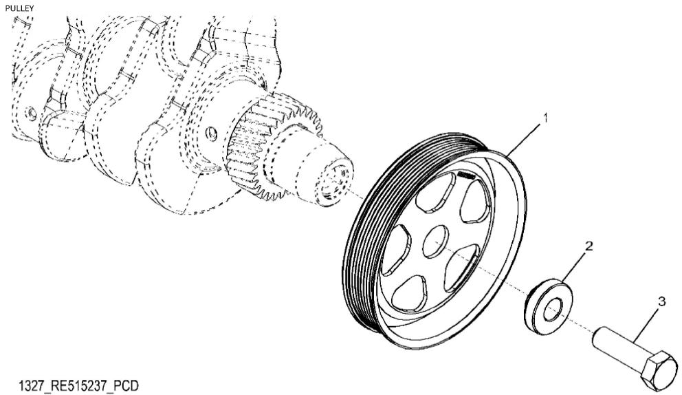
John Deere > Turf And Utility >TRACTOR >5100MH - TRACTOR >5100MH Tractor (Engine 4045HLV68,4045HLV70)(iT4)(North America Edition) >20 ENGINE 4045HLV70 >ST308624 - 1327 CRANKSHAFT PULLEY
