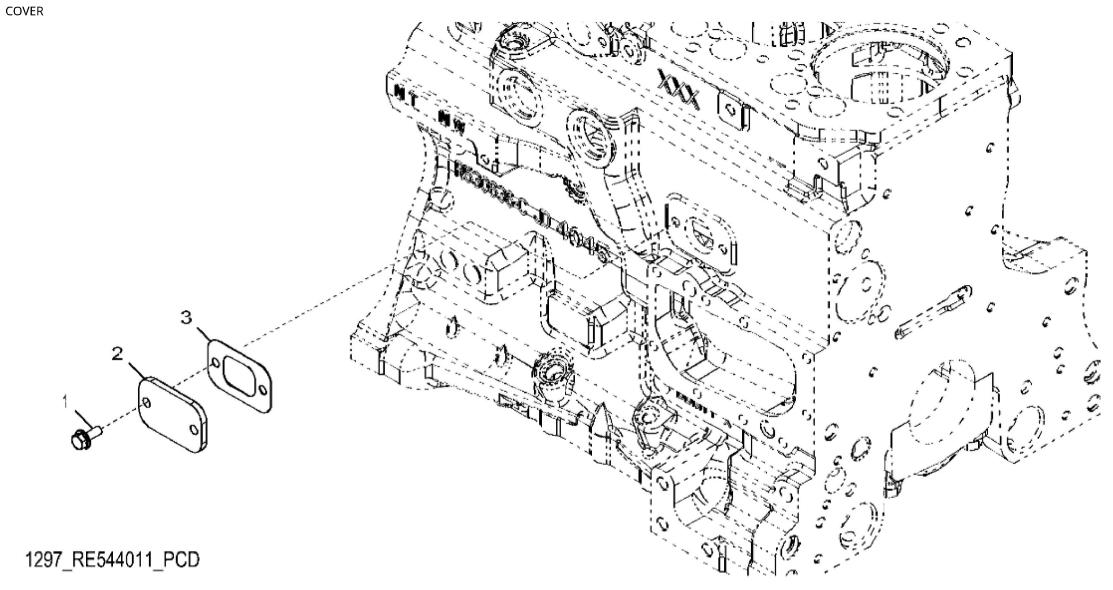
John Deere > Turf And Utility >TRACTOR >5100MH - TRACTOR >5100MH Tractor (Engine 4045HLV68,4045HLV70)(iT4)(North America Edition) >20 ENGINE 4045HLV70 >ST402282 - 1297 OIL FILLER COVER
