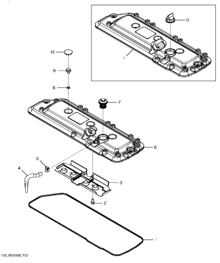
John Deere > Turf And Utility >TRACTOR >5100MH - TRACTOR >5100MH Tractor (Engine 4045HLV68,4045HLV70)(iT4)(North America Edition) >20 ENGINE 4045HLV70 >ST400926 - 1183 ROCKER ARM COVER
