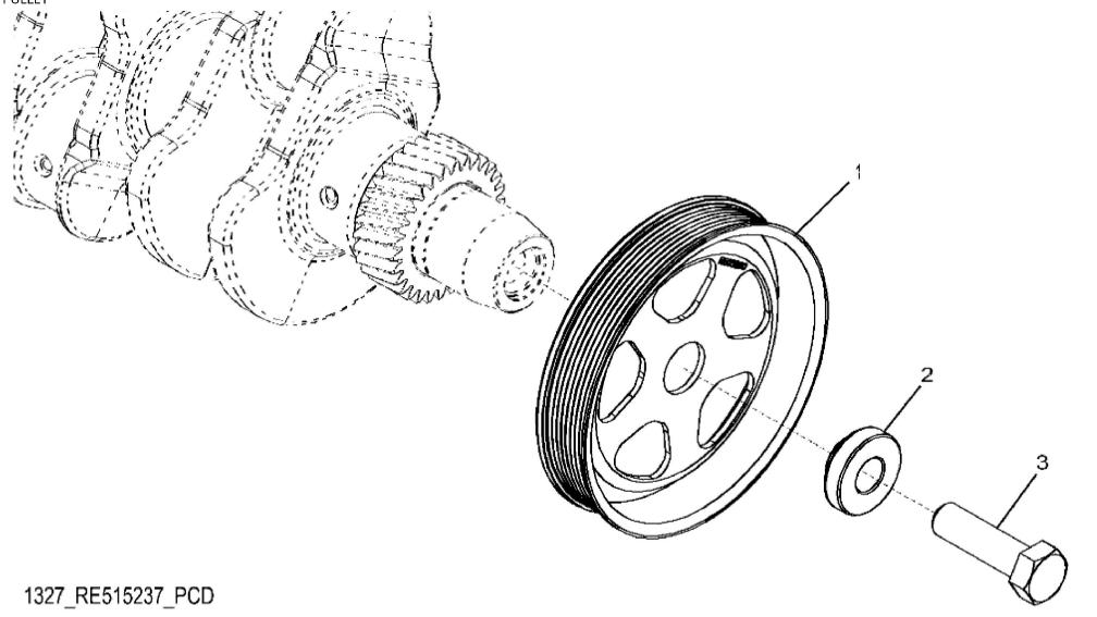
John Deere > Turf And Utility >TRACTOR >5115M - TRACTOR >5115M Tractor (Engine 4045HLV68,4045HLV70)(iT4)(North America Edition) >20 ENGINE 4045HLV70 >ST308624 - 1327 CRANKSHAFT PULLEY
