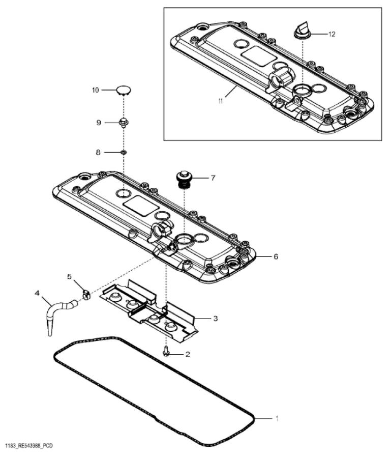
John Deere > Turf And Utility >TRACTOR >5115M - TRACTOR >5115M Tractor (Engine 4045HLV68,4045HLV70)(iT4)(North America Edition) >20 ENGINE 4045HLV70 >ST400926 - 1183 ROCKER ARM COVER
