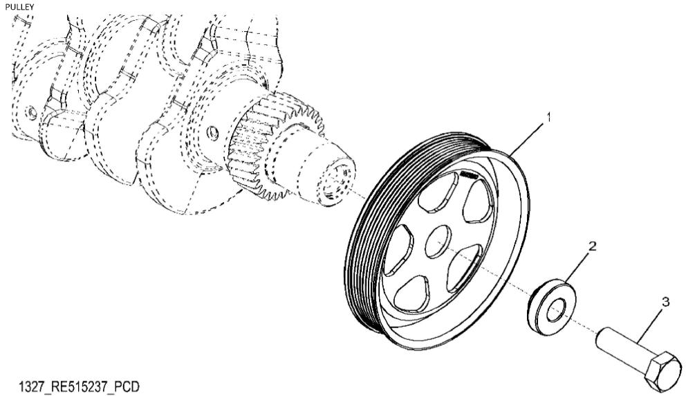
John Deere > Turf And Utility >TRACTOR >5115ML - TRACTOR >5115ML Tractor (Engine 4045HLV68,4045HLV70)(iT4)(North America Edition) >20 ENGINE 4045HLV70 >ST308624 - 1327 CRANKSHAFT PULLEY
