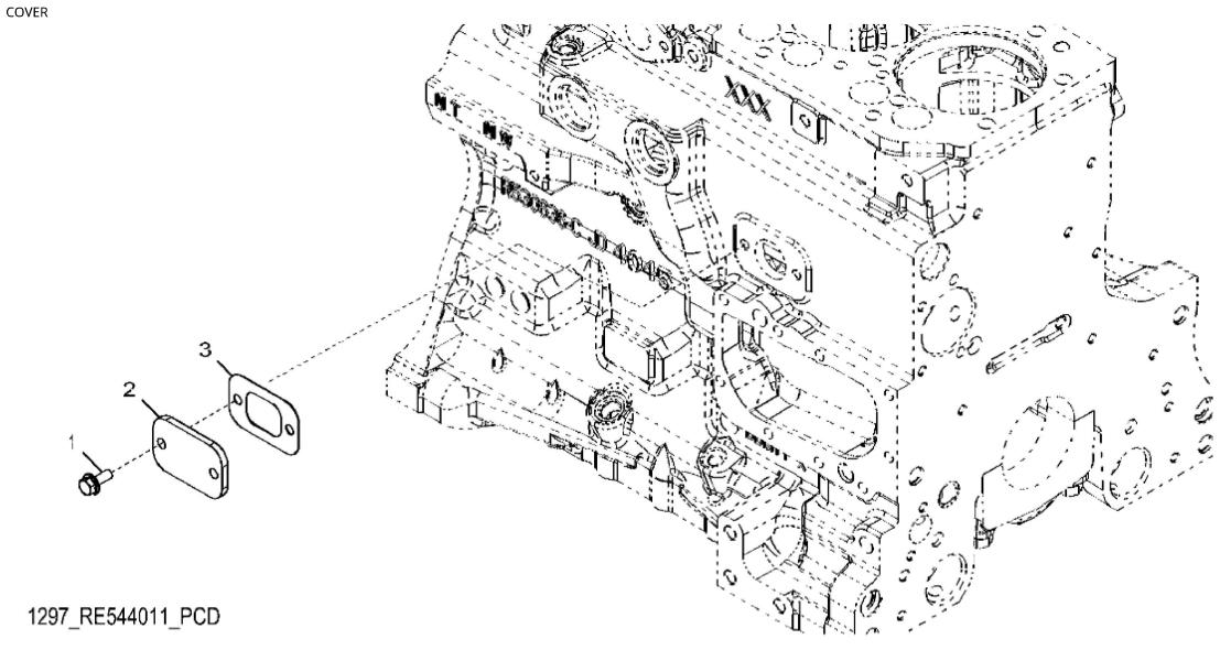
John Deere > Turf And Utility >TRACTOR >5115ML - TRACTOR >5115ML Tractor (Engine 4045HLV68,4045HLV70)(iT4)(North America Edition) >20 ENGINE 4045HLV70 >ST402282 - 1297 OIL FILLER COVER
