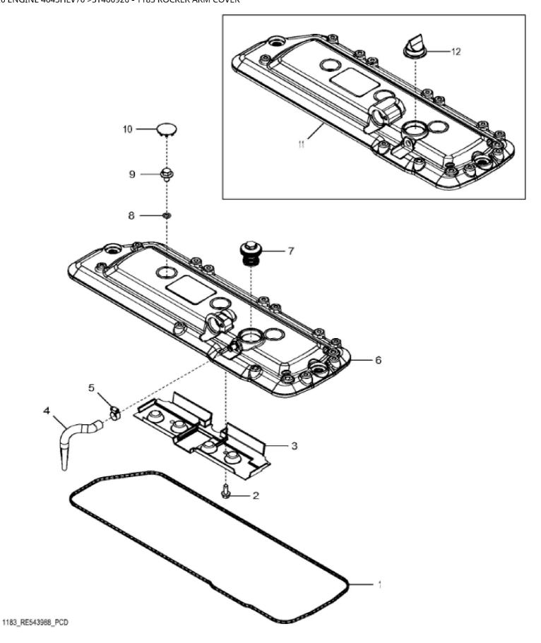
John Deere > Turf And Utility >TRACTOR >5115ML - TRACTOR >5115ML Tractor (Engine 4045HLV68,4045HLV70)(iT4)(North America Edition) >20 ENGINE 4045HLV70 >ST400926 - 1183 ROCKER ARM COVER
