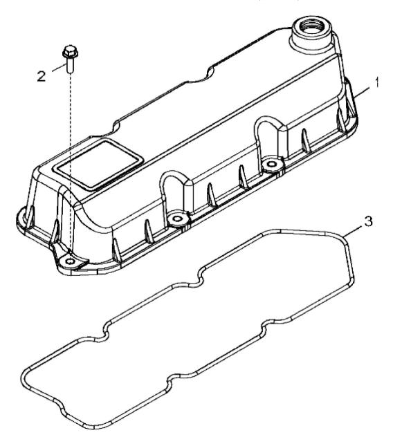
John Deere > Turf And Utility >TRACTOR >5065E - TRACTOR >5065E Tractor (IT4)(9X3 TSS Transmission W/ Cab)(12X12 PR Transmission W/ Cab and OOS) (For Europe, Australia, New Zealand, JDLA, Sub-Saharan Africa and Mexico) >20 ENGINE 3029HPY41-DZ100017 >ST757957 - 11AA ROCKER ARM COVER ( - XXXXXXX)
