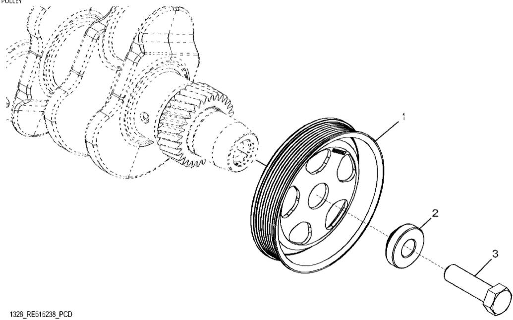
John Deere > Turf And Utility >TRACTOR >5100E - TRACTOR >5100E Tractor (Engine: 4045HLV69, iT4)(North American Edition) >20 ENGINE 4045HLV69-RE550040 >ST628039 - 1328 CRANKSHAFT PULLEY
