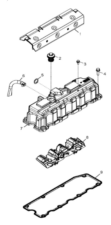
John Deere > Turf And Utility >TRACTOR >5075E - TRACTOR >5075E Tractor (Final Tier 4)(9X3 TSS Transmission and 12X12 PR Transmission)(North America Edition) >20 ENGINE 3029HPY61-RE571749 >ST756011 - 11AC VALVE COVER
