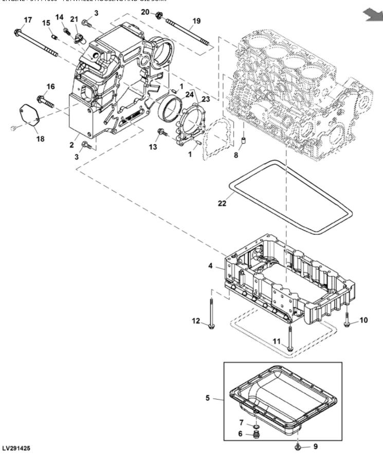
John Deere > Turf And Utility >TRACTOR, COMPACT UTILITY >4TNV86CHT - TRACTOR, COMPACT UTILITY >4066M Compact Utility Tractor >20 ENGINE >ST771060 - FLYWHEEL HOUSING AND OIL SUMP
