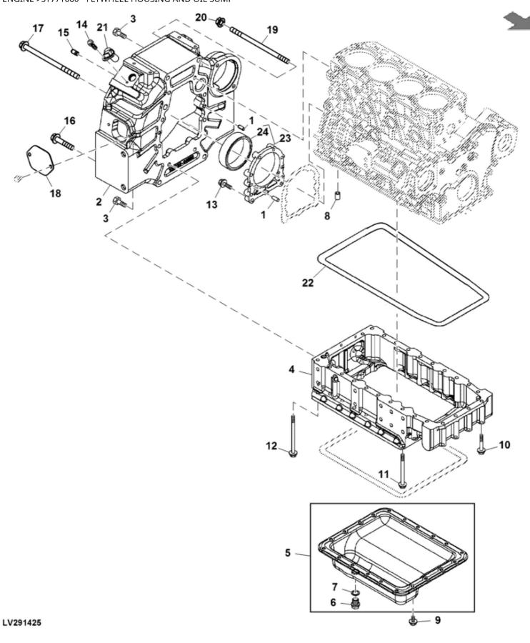
John Deere > Turf And Utility >TRACTOR, COMPACT UTILITY >4TNV86CHT - TRACTOR, COMPACT UTILITY >4066R Compact Utility Tractor >20 ENGINE >ST771060 - FLYWHEEL HOUSING AND OIL SUMP
