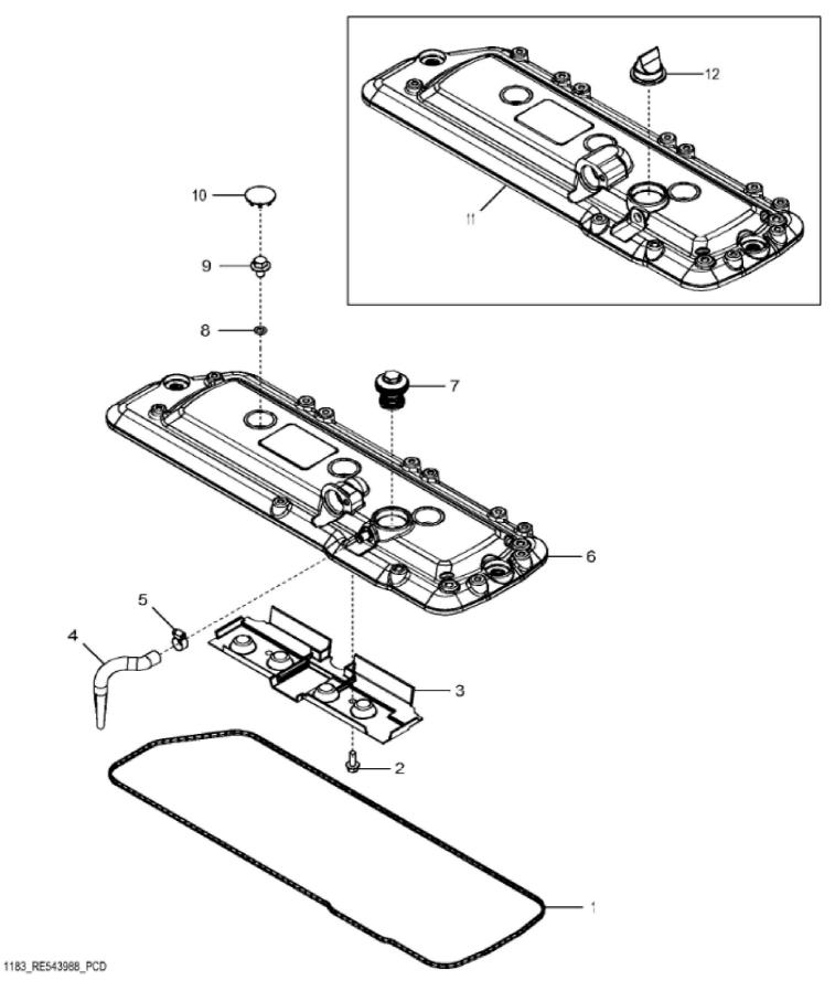
John Deere > Turf And Utility >TRACTOR >5085M - TRACTOR >5085M Tractor (S.N. 500001-)(IT4)(Engine 4045HLV70)(Europe Edition) >20 ENGINE 4045HLV70 >ST400926 - 1183 ROCKER ARM COVER
