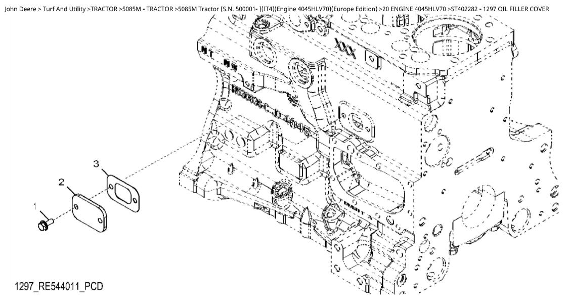
John Deere > Turf And Utility >TRACTOR >5085M - TRACTOR >5085M Tractor (S.N. 500001-)(IT4)(Engine 4045HLV70)(Europe Edition) >20 ENGINE 4045HLV70 >ST402282 - 1297 OIL FILLER COVER
