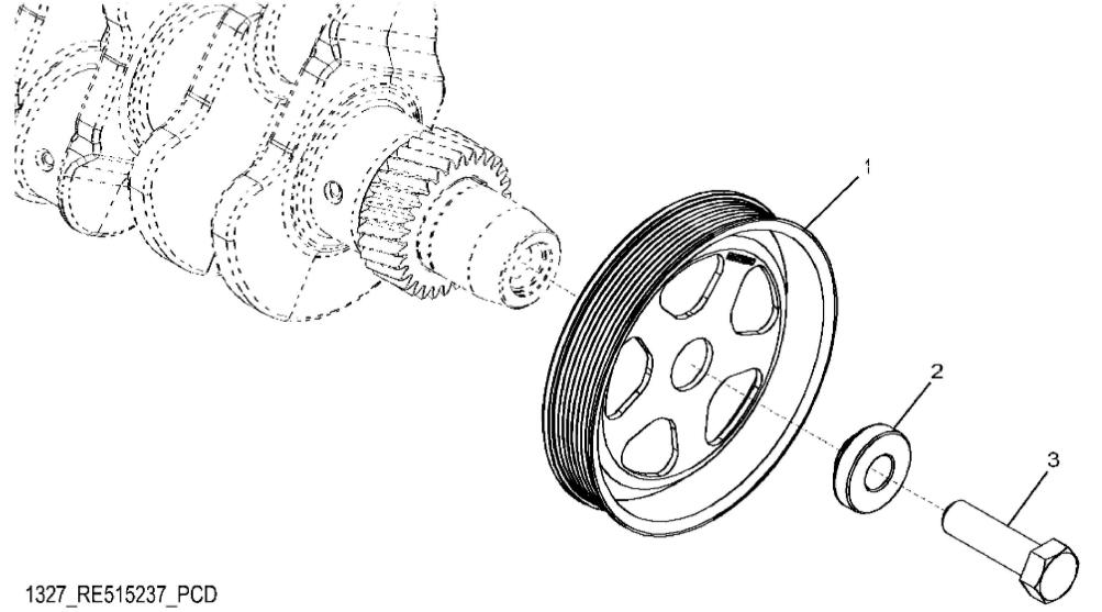
John Deere > Turf And Utility >TRACTOR >5100M - TRACTOR >5100M Tractor (S.N. 500001-)(IT4)(Engine 4045HLV70)(Europe Edition) >20 ENGINE 4045HLV70 >ST308624 - 1327 CRANKSHAFT PULLEY
