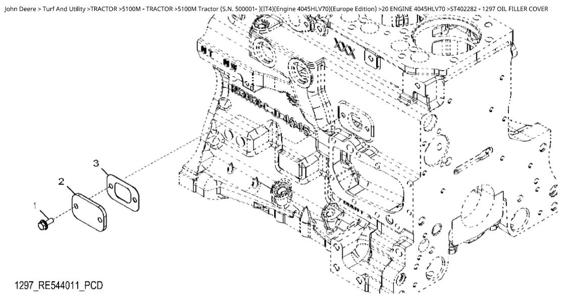
John Deere > Turf And Utility > TRACTOR > 5100M - TRACTOR > 5100M Tractor (S.N. 500001-)(IT4)(Engine 4045HLV70)(Europe Edition) > 20 ENGINE 4045HLV70 > ST402282 - 1297 OIL FILLER COVER
